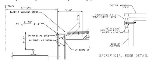
The dimension between the track centerline and the edge of the "gap filler" after installation should be 5'4.85" meaning the gap filler must protrude 5.65" from the face of the platform. The length of each piece of platform gap filler should be such that it would minimize the number of pieces required to install the gap filler to the entire length of each platform.
