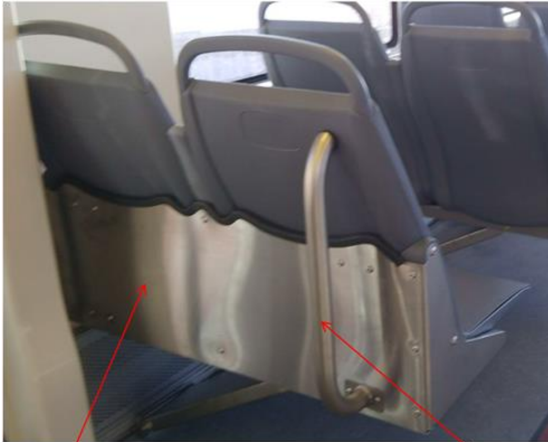
Barrier Seat Structure
