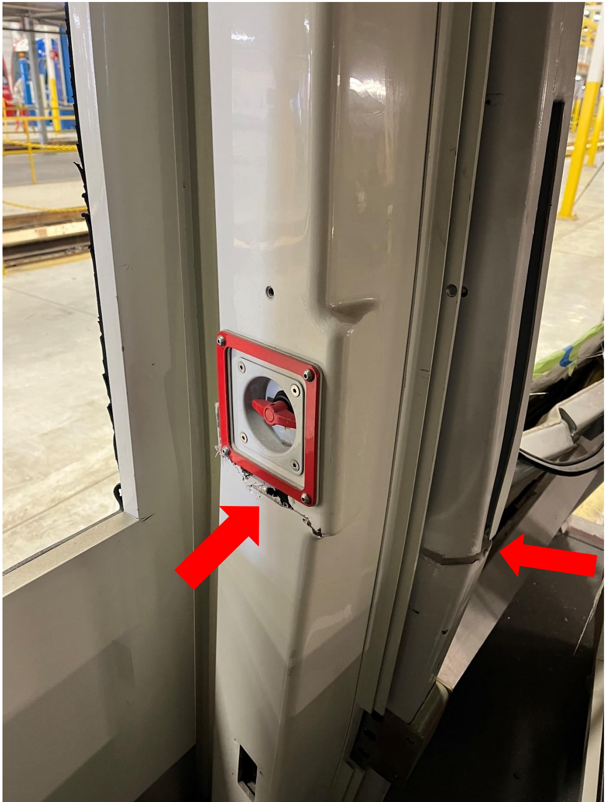
RH Side Door 1 Interior Frame/Trim Damaged Adjacent to Window in Between Door 1 and 2
