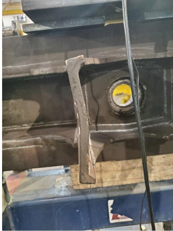
Figure 6: Damaged Bolster Lateral Bumper Stop.
