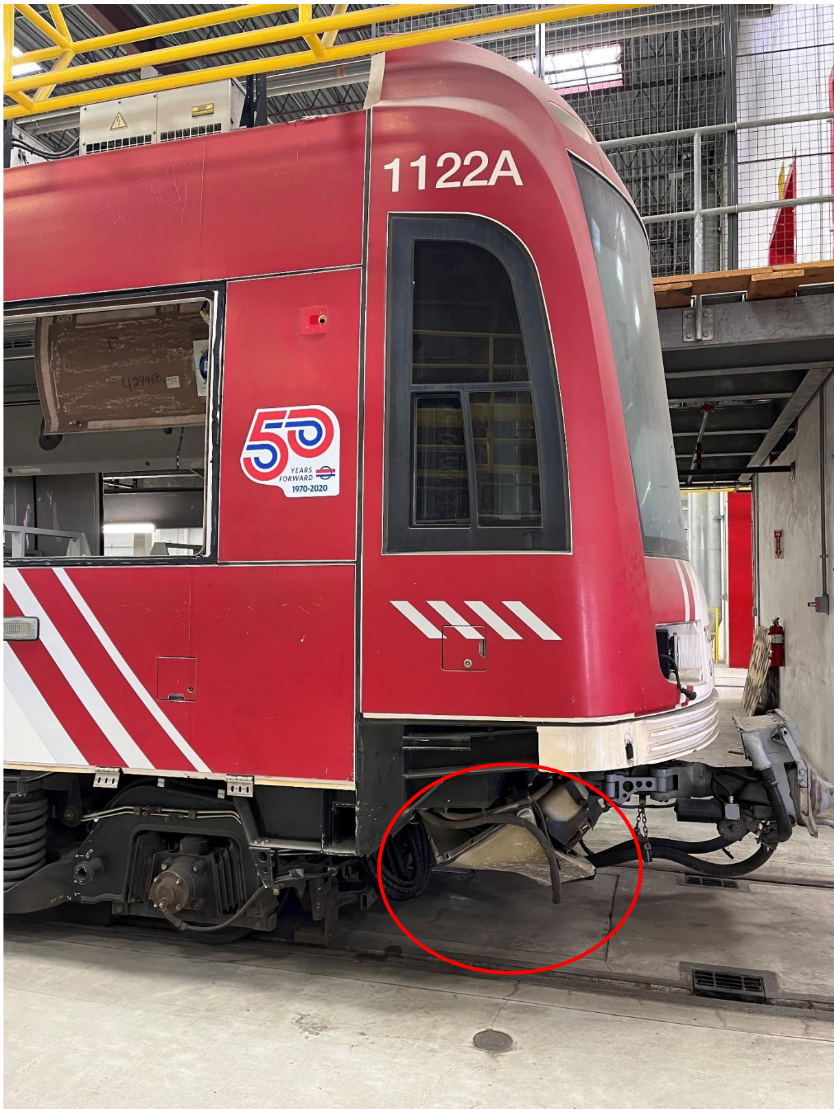
RH side 162 Box – damaged, including windshield washer reservoir
