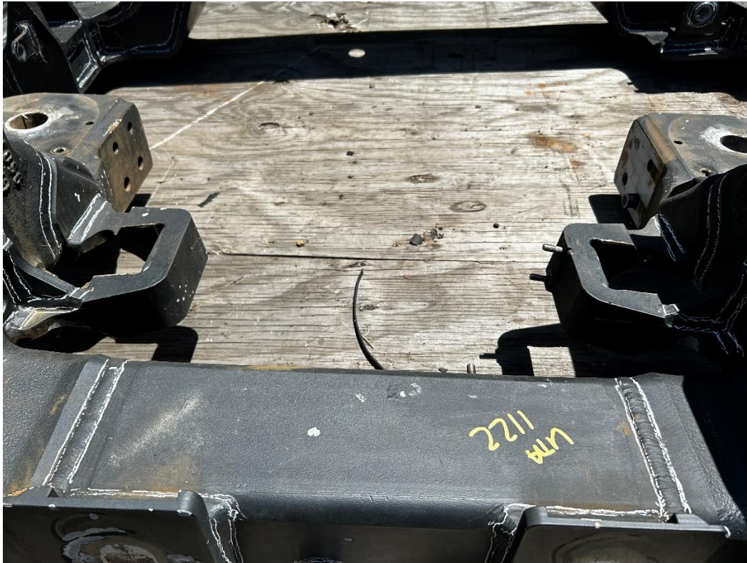
Figure 2: Damaged track brake brackets.
