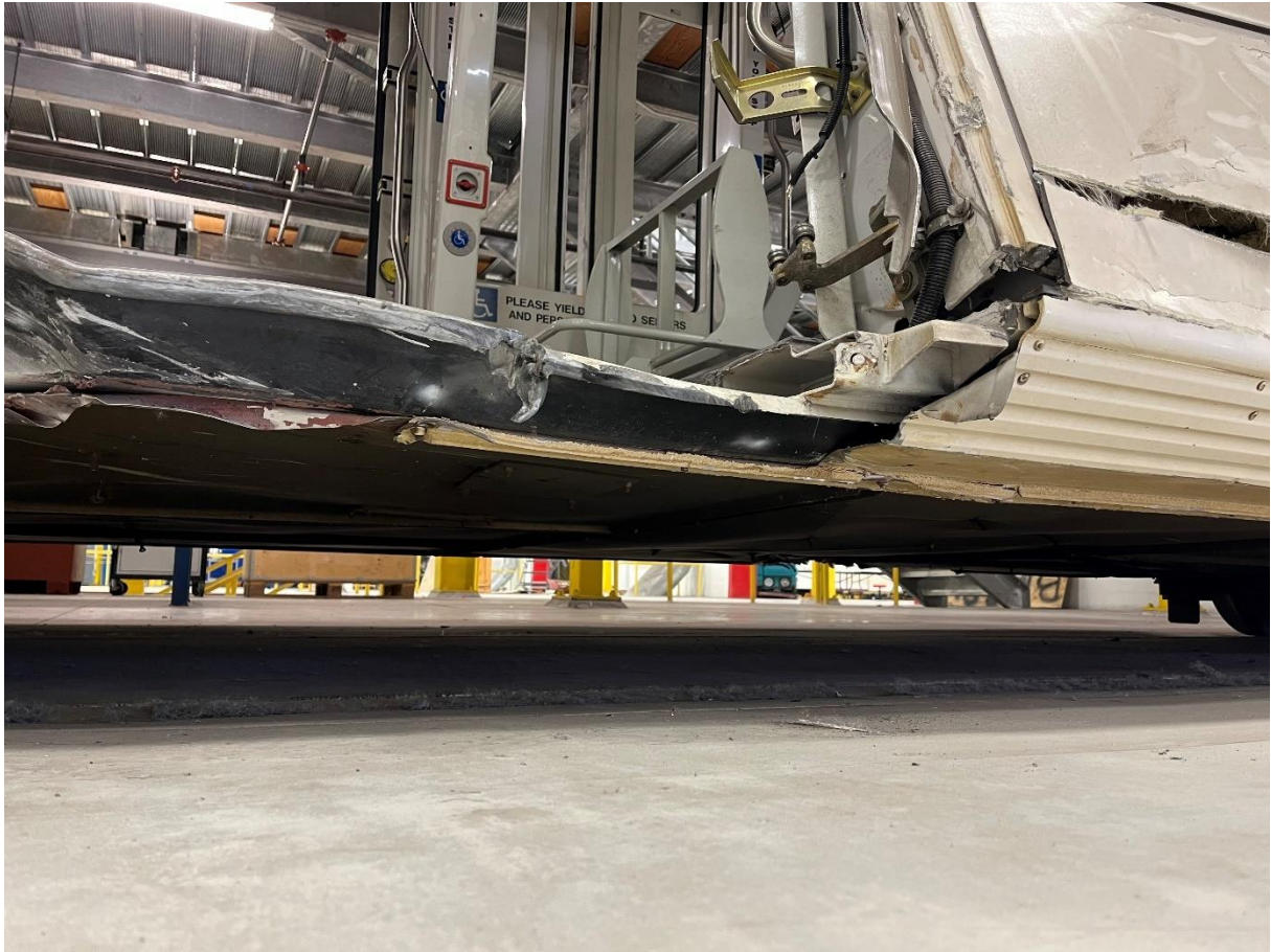
Door 2 Ramp/Threshold Impact Side
