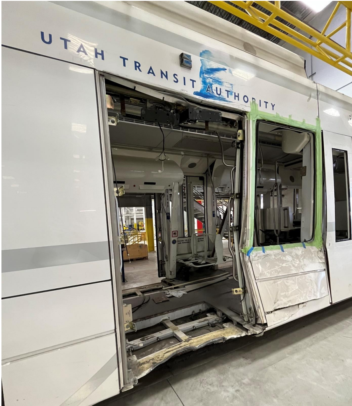
Right Hand Side Door 2 Primary Impact Area of "A" Car
