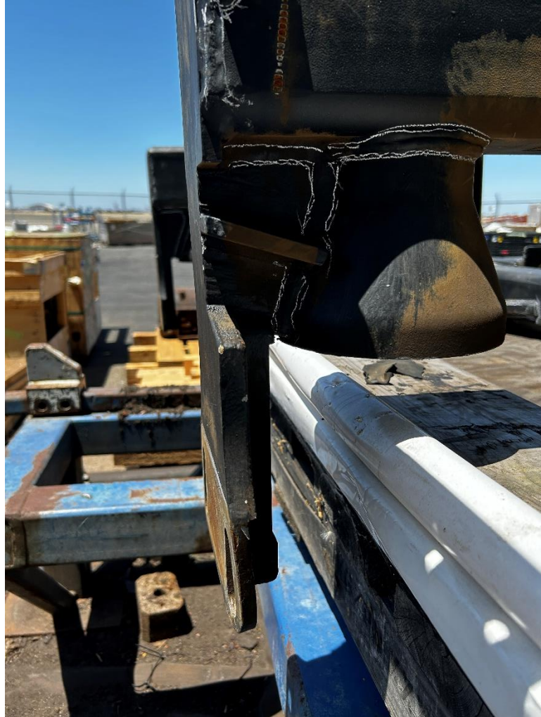
Figure 1: Track Clearer Bent Lifting Device Bracket
