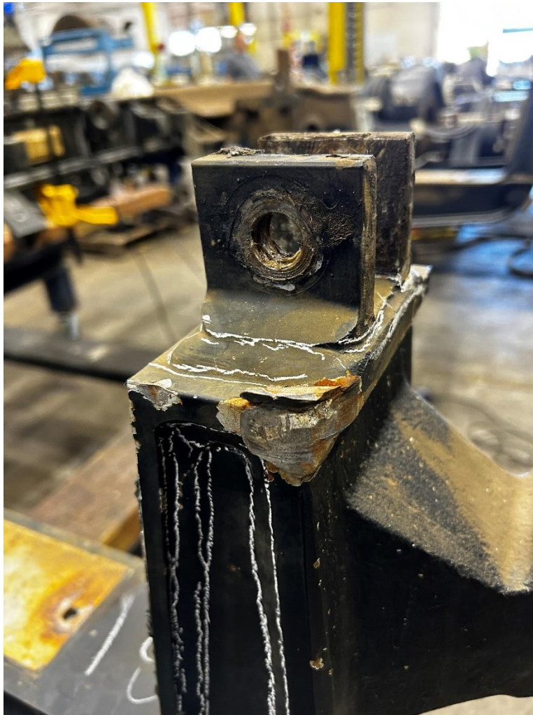
Figure 8: Damage to the corner of the frame.
