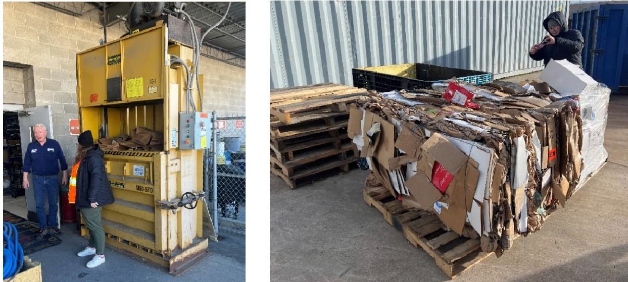
Figure 5-13. Cardboard Baler and Finished Bale at Meadowbrook
