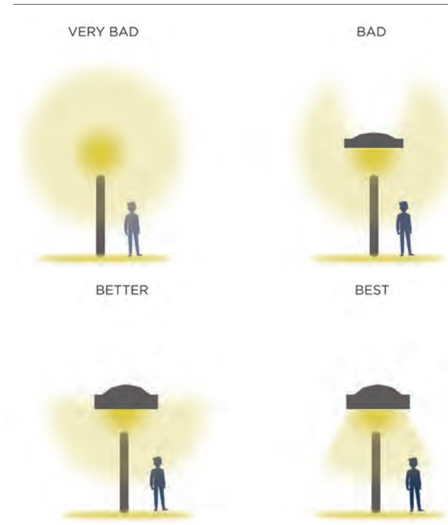
FIGURE 6.4: PROPER LIGHTING ILLUSTRATION
